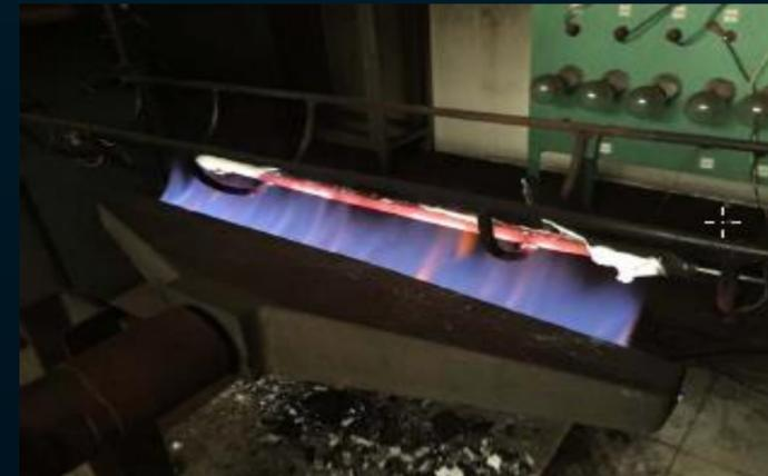
**Optical cable combustion test**
